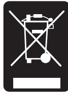
Fig. 1.4: Product labeling in accordance with EN 50419
